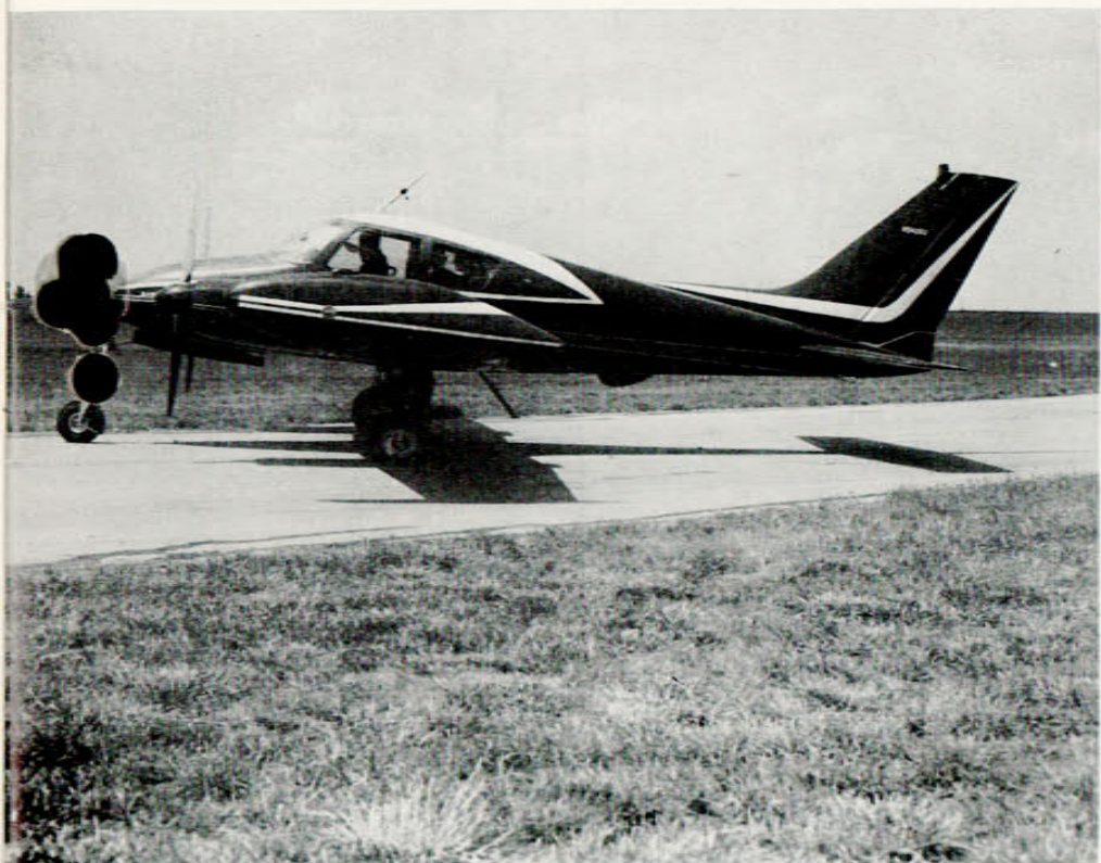
Dramatic new styling of Cessna's 1960 Model 310D is illustrated with the exterior design of the swept vertical fin. The 310D is powered by dual Continental 260 h.p. engines with fuel injection, providing the airplane with a cruising speed of 220 m.p.h. and a 440 foot per minute rate of climb on only one engine.
