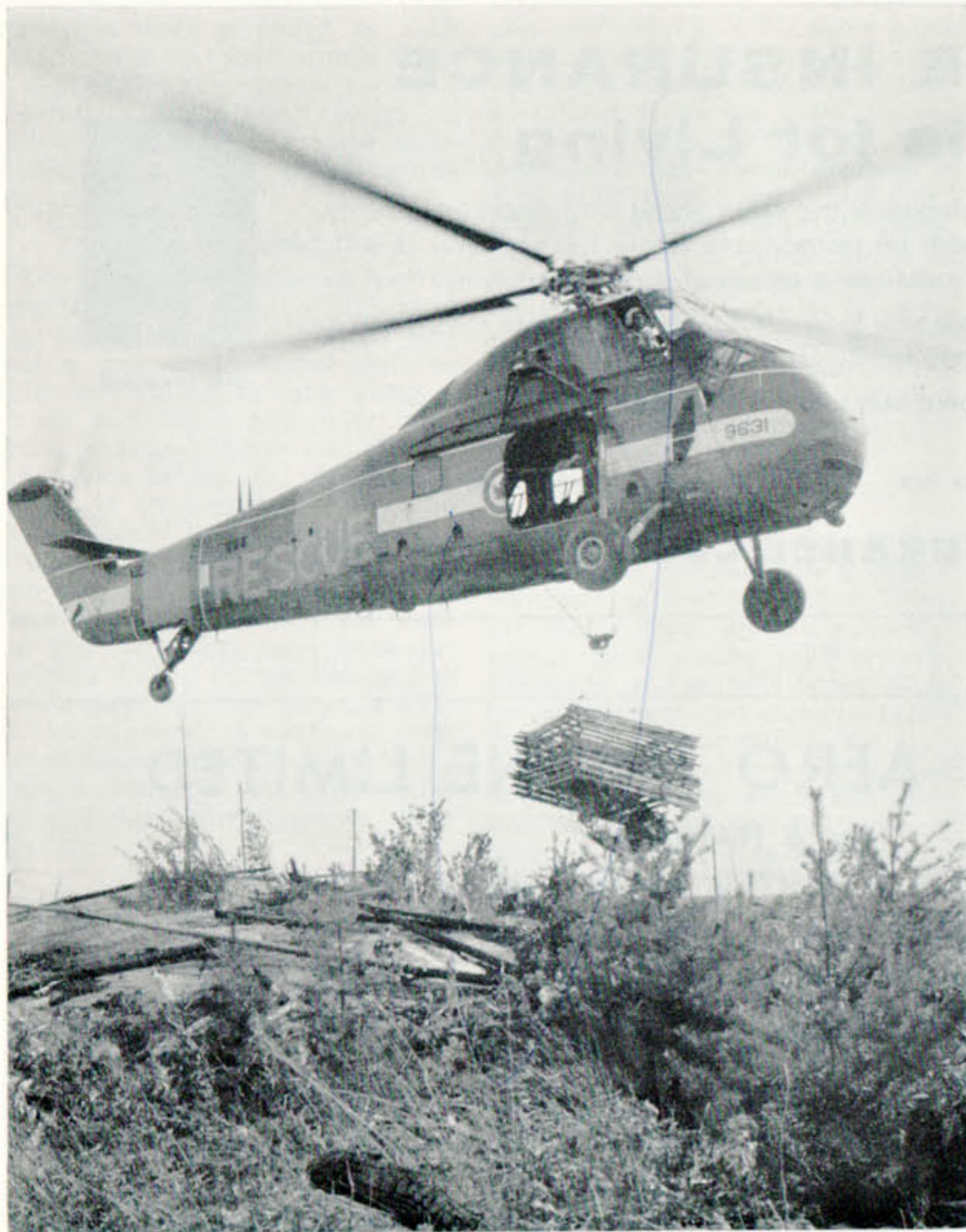
The H34 Helicopter — used extensively by 111 Composite Unit. Besides being invaluable in search and rescue the H34 is excellent for moving cargo from difficult locations.
