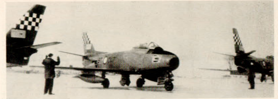
Canadian airmen at Metz, France, have solved the problem of clearing ice off Sabre jets during the cold weather. The ice-coated Sabre is slowly taxied between the tails of two other jets and the heat from the exhausts quickly melts the ice.
