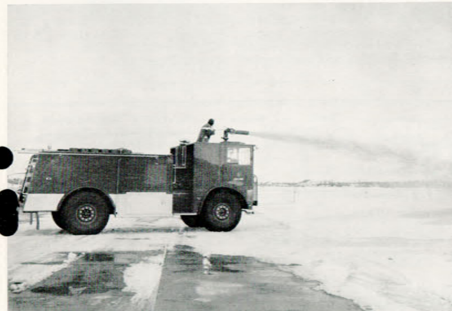
The G23 shooting foam through its manually operated turret.
