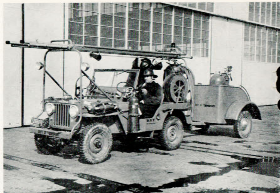
The Department of Transport use a jeep and trailer manned by a volunteer crew for combatting civilian aircraft fires.
