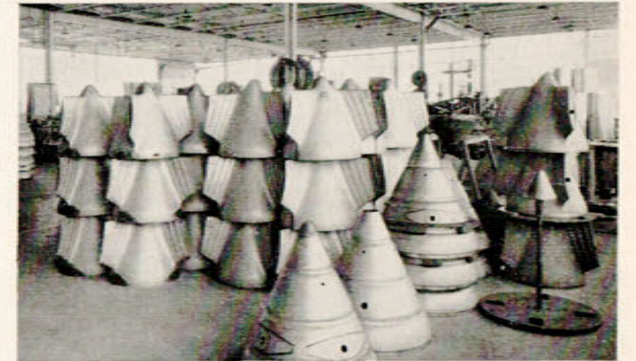
Among the Company's contracts has been the manufacture of engine components for the Orenda and Nene turbojets. Such production has served to emphasize the capacity for highly skilled, close tolerance sheet metal work.
