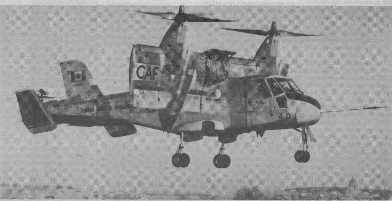
The CL-84 Tiltwing V/STOL was developed in the mid-sixties for transport and search and rescue evaluation. Four aircraft were built prior to termination of the experimental program in 1974, one sample being donated to the National Aviation Collection and one to the Western Canada Aviation Museum in October 1985.
