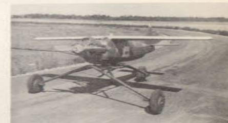
PL-65160—TAKE-OFF—One of the RCAF's new Radio controlled planes is caught in flight just after being launched. The radioplane, at this time, is controlled by the ground pilot.
