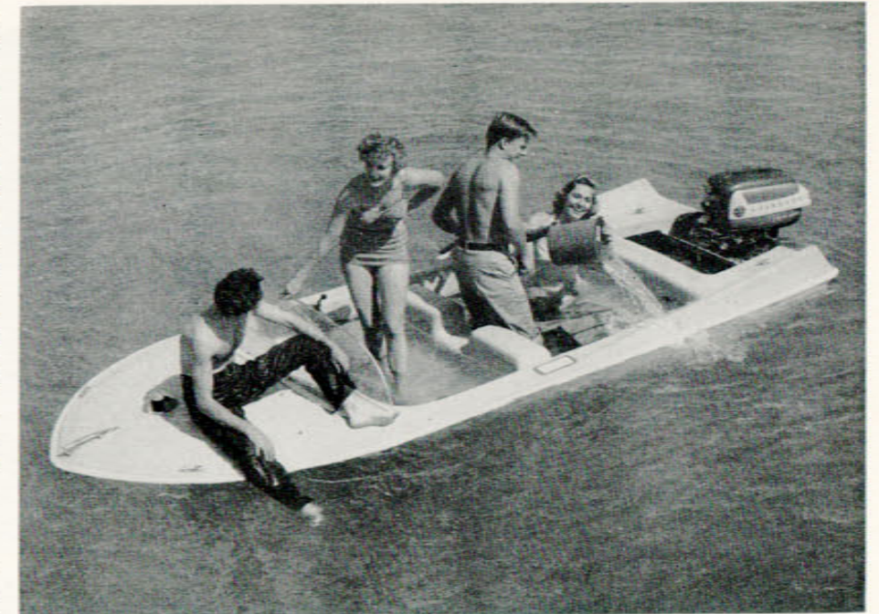
Here's a boat that won't sink, even when it's swamped. The boat is made of Expanded Royalite, a new material developed by United States Rubber Co.
