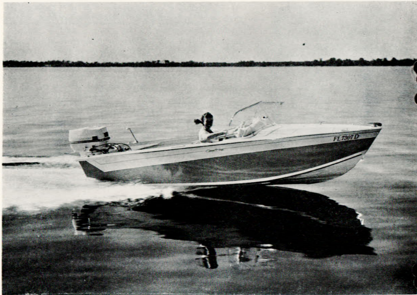
This trim, 16-foot Carter Craft runabout features the unsinkable new material known as Expanded Royalite, developed by United States Rubber Co. The rubber company forms hulls and decks to the specifications of boat manufacturers. Carter Craft, of Panama City, Fla., is the latest firm to utilize the material in its boats.
