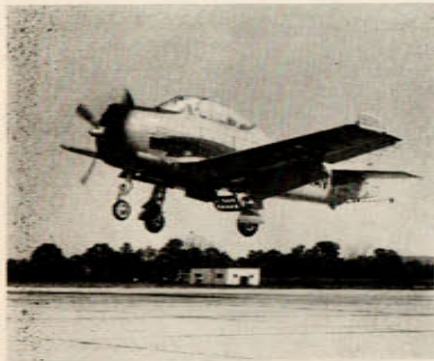
FIRST FLIGHT—NORTH AMERICAN NAVY T-28C The new North American Navy T-28C trainer comes in for a landing on its first flight at the company's Columbus, Ohio Division. Major changes in "C" model is addition of arresting hook and barrier gear for carrier operation. The first "C" was flown and accepted by the U.S. Navy 24 hours after completion by North American.
