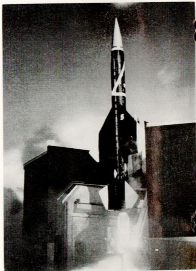
Bomarc at the instant of launch from its platform within its storage, check-out and launching cell.
