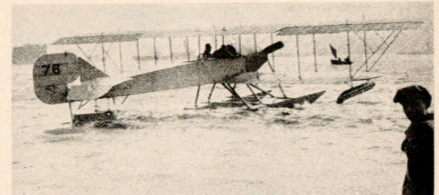
The Short S.41 which carried four 100-lb. bombs. S.41s took part in raids on Cuxhaven and Wilhelmshaven in 1941; they had a crew of two and were powered by a Canton Unne 200-h.p. engine.
