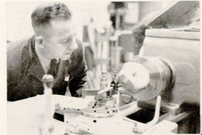
Cpl. "Phil" Scarrow (above) and LAC J. Bullied are two of the machinists of Station Workshops. Cpl. Scarrow, who is also a percussionist with the Station Band, is operating the lathe with a "turret" attachment, used for production work.
