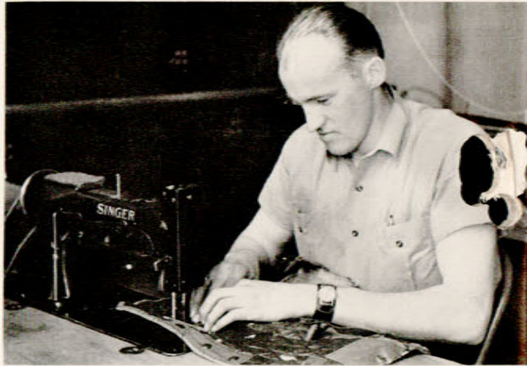
"Made to measure" . . . LAC R. Wilkinson is manufacturing a part of the leatherette upholstery for a Dakota.
