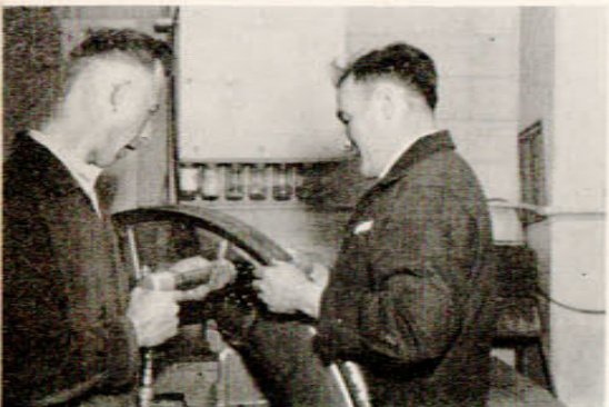
"A little patch should do the trick." LAC A. M. Jensen (left), and Cpl. J. R. Lloyd repair an Expeditor firewall.
