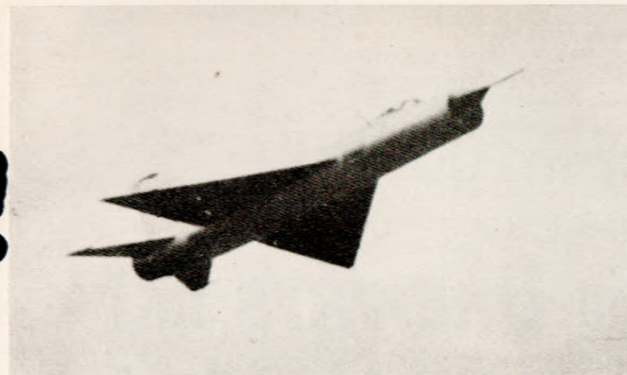
One of three Sukhoi experimental delta fighters that flew at the Tushino air show. This model shows radome nose, chin air intake which may be bifurcated and 30 mm. cannon gunport just forward of leading edge of delta wing. Note thin delta wing and low set horizontal tail.
