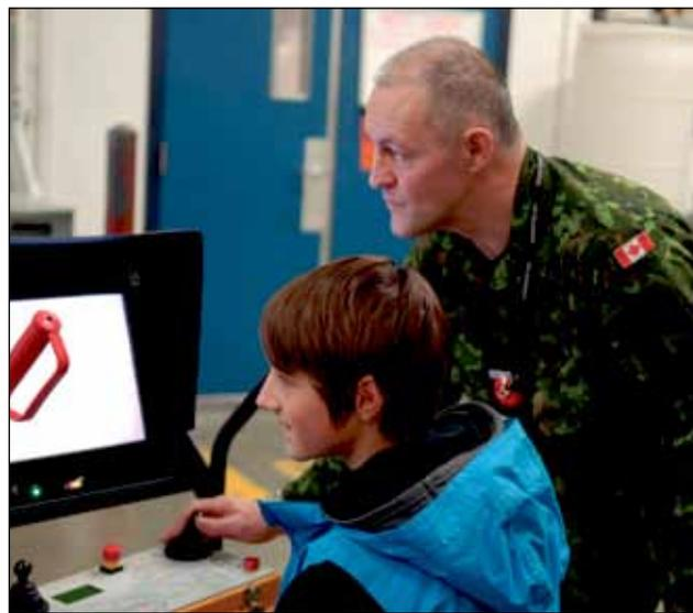
A Corporal with 435 Squadron showing a student how to operate TEO, the telerob Explosive Ordnance Disposal and Observation Robot, from the remote control panel. Photo: Martin Zeilig
