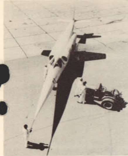
Recently released photograph of the USAF's X-3 research aircraft, nicknamed the "Flying Stiletto" and designed to fly 2,000 m.p.h. Fuselage is 66 feet, nine inches long; the wing span is 22 feet, eight inches.
