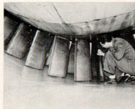
A Boeing Airplane Company wind tunnel engineer inspects the new laminated glass-cloth fan blades recently installed in the company's transonic wind tunnel at Seattle. These blades are believed to be the first of this type used in any wind tunnel. Each of the new blades weighs only 50 pounds, but is capable of sustaining forces of 19 tons and temperatures of 200 degrees Fahrenheit encountered when the tunnel is operating at high speeds.
