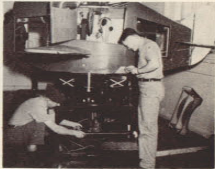
No. 2. LAC C. K. Judd and Cpl. R. Cowley doing a 50 hour inspection on one of the Link Trainers.
