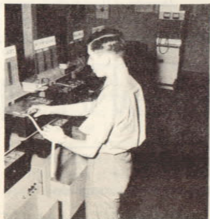
ACI Roy Surette relays the tape to Ottawa on the transmitter distributor—the final step in the actual transmission of the signal.
