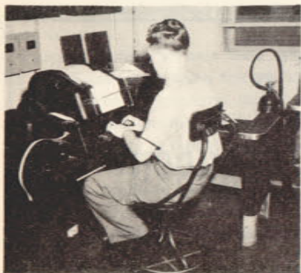
ACI Gordon Murdock transforms the signal to a "Chad" tape on Model 19 Perforator.
