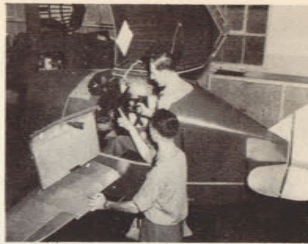
No. 1. F/O L. Klein (in Link) being shown workings of instrument landing system (I.L.S.) by F/O D. Button.
