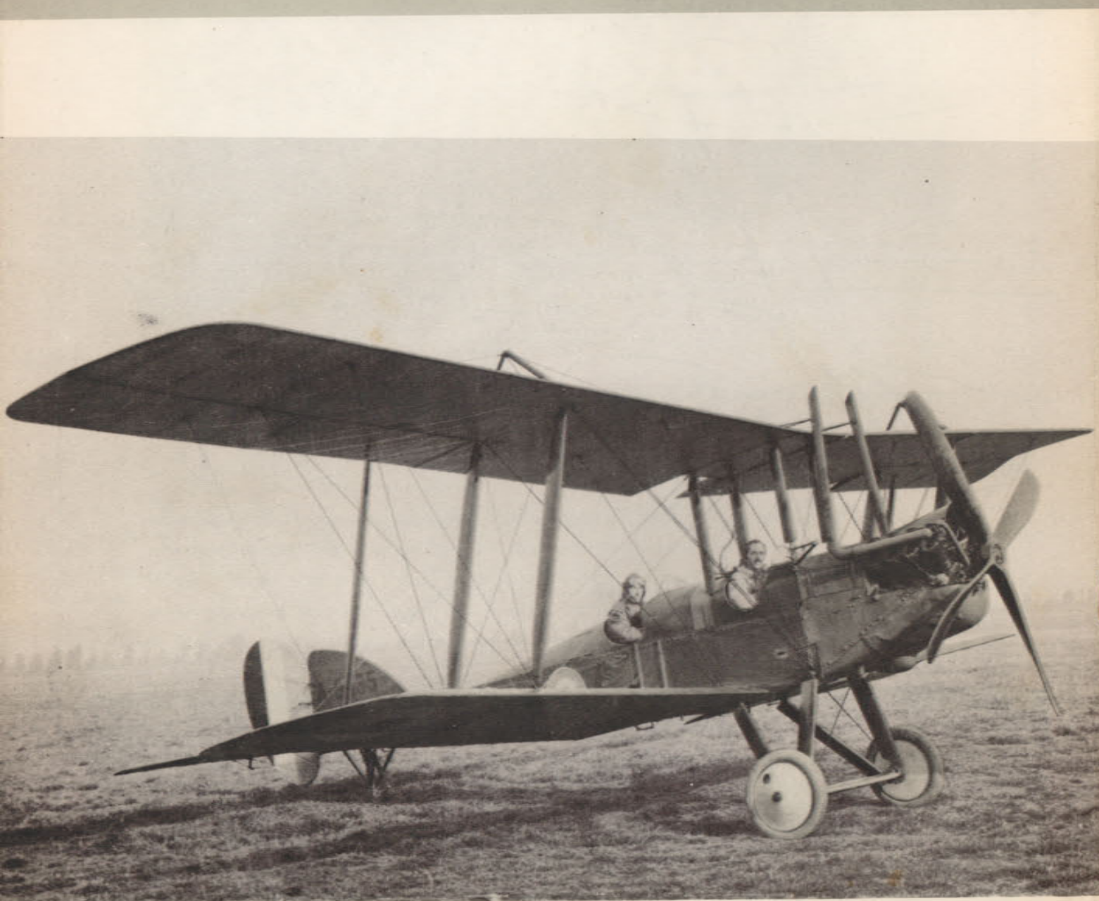
R.E. 8 Reconnaissance Experimental 90 h.p. Royal Aircraft Factory Engine.
