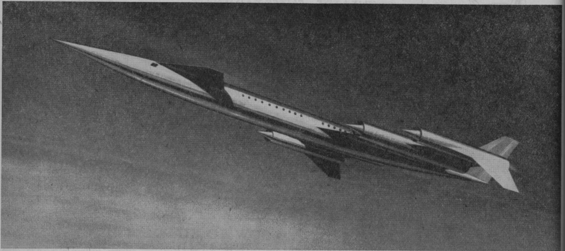
A 2000-mph supersonic transport prototype can be flying within five years and an operational version in regular airline service by 1973, according to a Lockheed-California engineering research executive. Pictured is a recent Lockheed SST concept, one of many under study by company engineers. The operational SST, built of titanium and special steels to withstand the 625-725 degree Fahrenheit temperatures reached at three times the speed of sound, could carry 120-125 passengers from New
