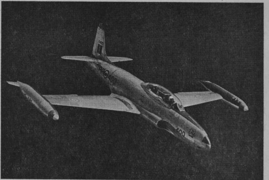
The T-33 Silver Star jet trainer has been in use by the R.C.A.F. for ten years. The "T-bird" was used extensively in the training of NATO aircrew. A complete engine change may be carried out on a T-33 in 30 minutes.
